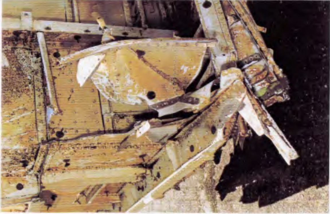
Fig. 12 Detail of the STA 395 bulkhead (RH-side)
